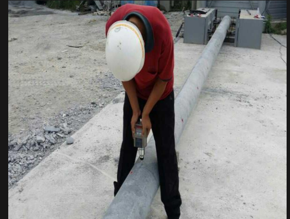
Compressive strength test
