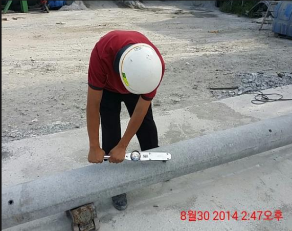
Step nut test for toehold
